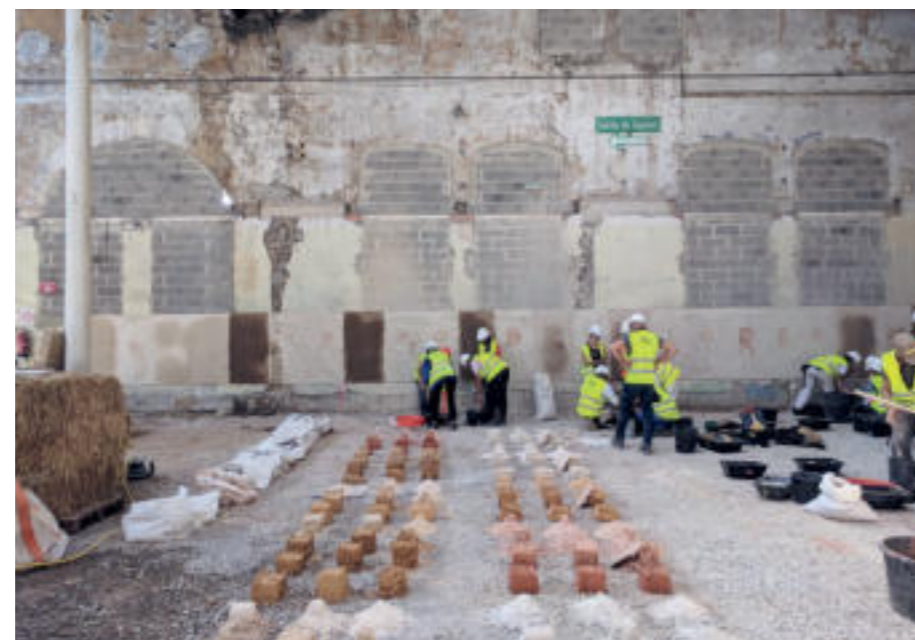
Experimentieren und Entwickeln lokaler Ressourcen zu Bauprodukten. Experimentation and development of local resources into building products.
